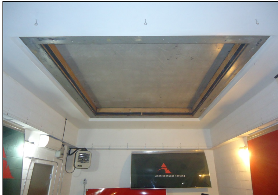
Receive Room View of Test Specimen Installation
