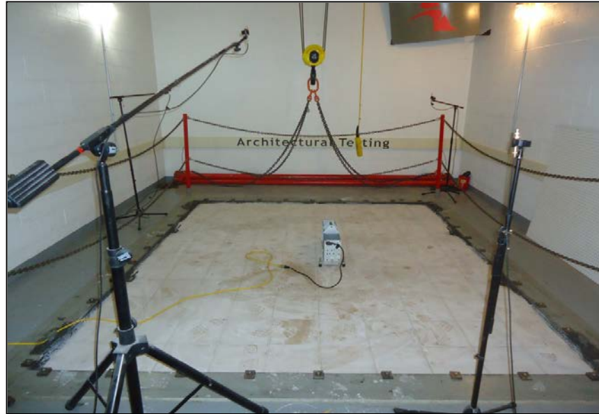
Source Room View of Test Specimen Installation
